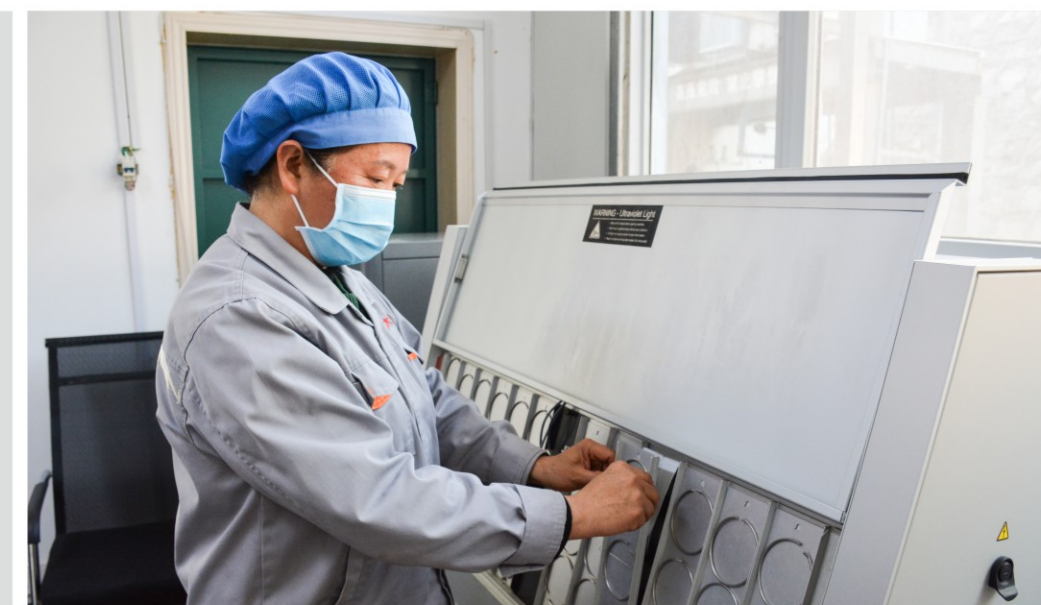
抗老比测试 Ageing resistance test
